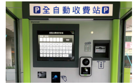
Intercom as a voice access point for service and emergency
